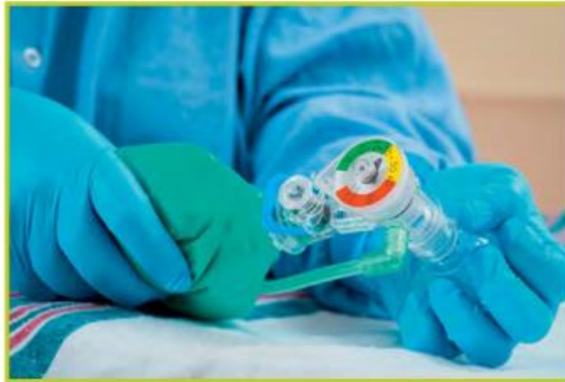
Figure 4A.6. Testing a flow-inflating bag
