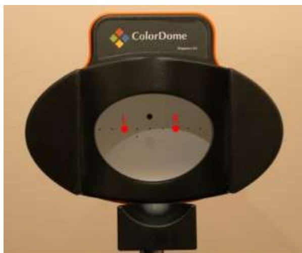
Fig. 52. Ganzfeld showing Left/Right fixation points for EOG.
